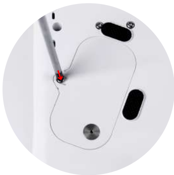
① Loosen the base cover screw
