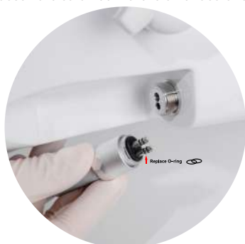
③ Replace the o-ring or install a new cord
