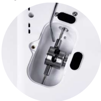
③ Blow away the powder left in the pinch valve chamber with an air gun.
